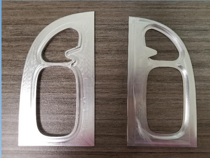
Machined from 6061 Aluminum
