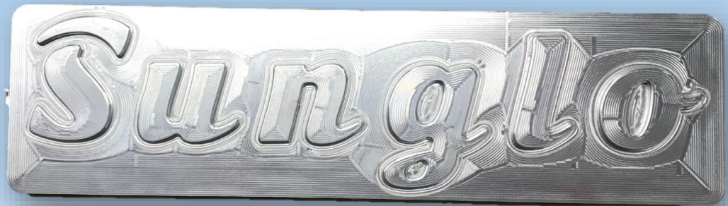
Machined from 6061 Aluminum
