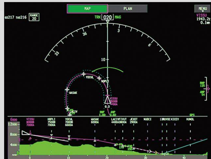
Left, Center – implementation of runway collision avoidance on Boeing's airplanes, Right, lower portion of image shows implementation of Vertical Situation Display (VSD)
